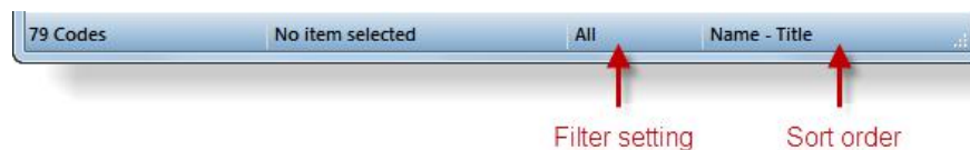
Figure 340: Indication of filter setting and sort order in the status bar of object managers
